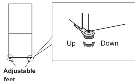
1. Lift up the bottom of the refrigerator slightly and turn the adjustable feet.
